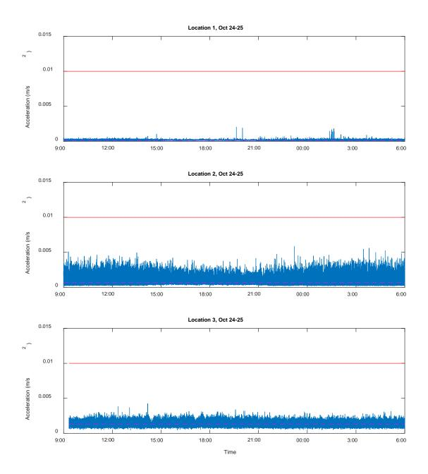
Figure 1: RMS particle accelerations at Location 1, 2 and 3 on October 24-25, 2017. The magenta dash line represents the mean baseline RMS particle acceleration calculated from October 5 to 16 at each location. The red line shows the 0.01 m/s<sup>2</sup> threshold of the RMS particle acceleration.
